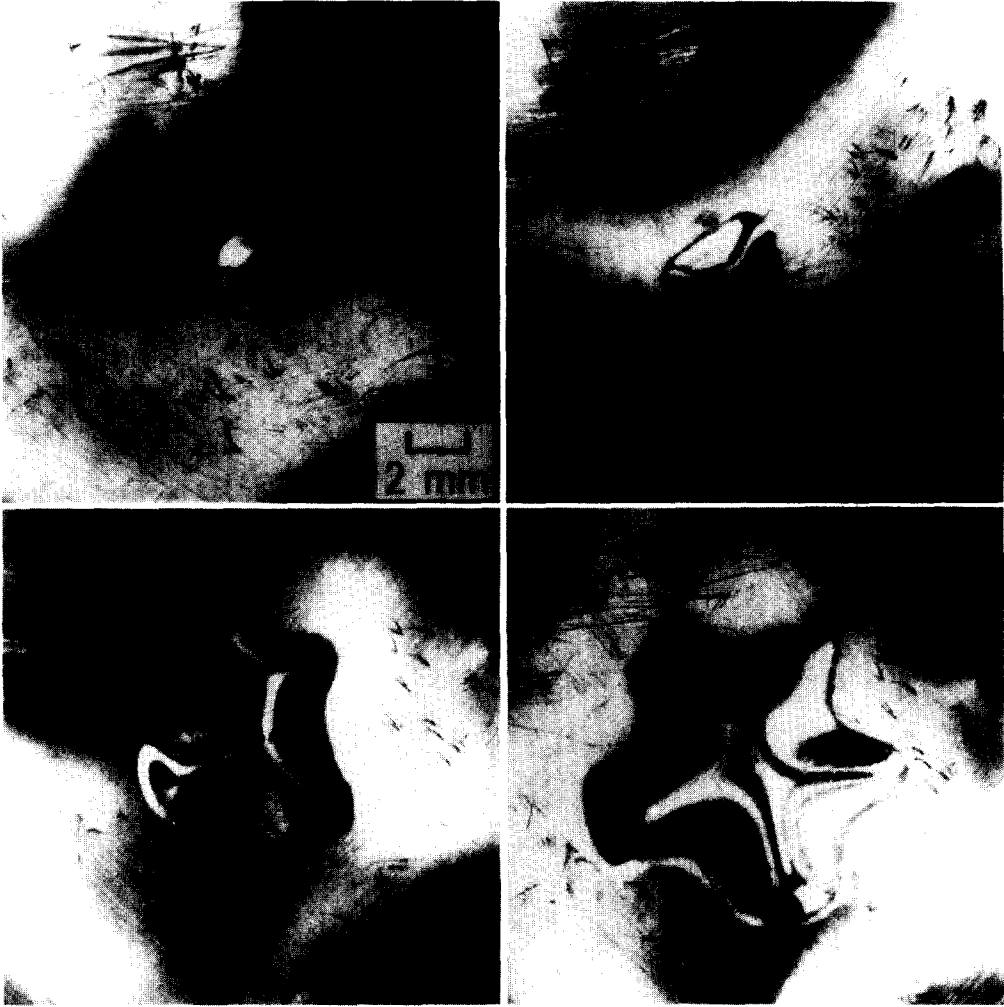
Fig. 12. A sequence of photographs showing the development of the shape of the mica-resin interface. The delamination was propagated by means of a point load, and there was a residual stress in the film.
